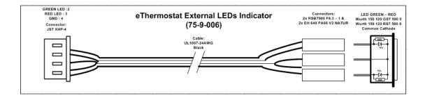
The External Led Indicator Option can be connected to the Port B of the eThermostat. After the connection the eThermostat automatically recognizes the options and changes their own operation.
